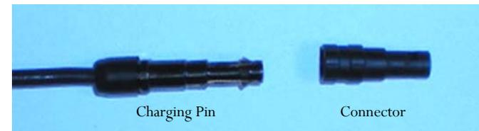
Figure 1: Components of robot charging system
