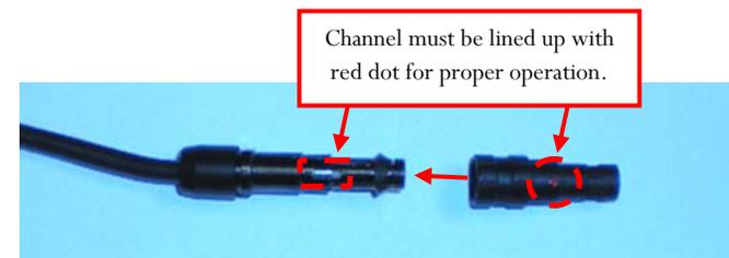
Figure 2: Correct alignment of red dot on Connector and channel on pin
