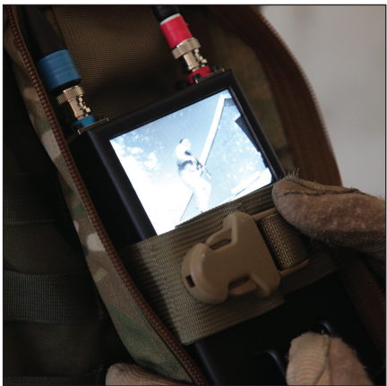
Robot transmits video 300 feet (91 meters)outdoors
